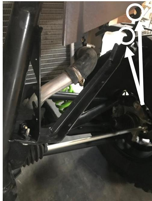
13. Fasten each headlight to the vehicle with the provided  $\frac{1}{4}$ " bolts, washers, and nuts in the configuration as shown below. The external faces of the headlight bracket are placed onto the internal faces of the headlight opening. Mount the grill temporarily to check the headlight clearance and remove to adjust. Once satisfied, remove the grill and tighten the fasteners.
