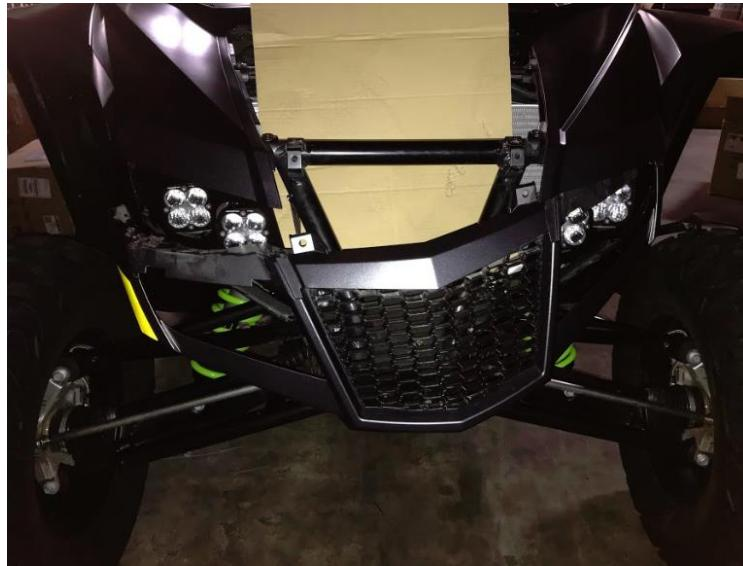
6. Disconnect the headlight plugs (2 each side). Locate the headlight adjuster knob on the inboard side of both headlights and remove. Now, using the needle-nose pliers, remove the four silver retaining clips on each of the headlight mounting points.
